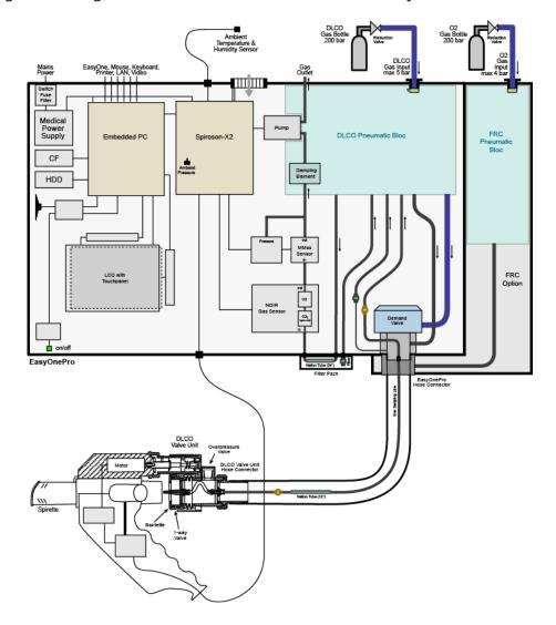
Sensors for flow, gas-composition, and pressure are located at two different positions: The so-called "main-stream" sensors are located near the patient's mouth in the hand-held unit; the "side-stream" sensors are located within the EOPL device. A sampling tube moves gas at
