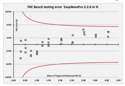
The two red lines in the diagram above indicate the  $\pm 5\%$  error in FRC, including an error of 1 mm in water level (water level of the lung model measured visually). Only measurements above 0.75 L FRC have been performed, since the error from the water level measurements exceeds 50% of the 5% error margin.
